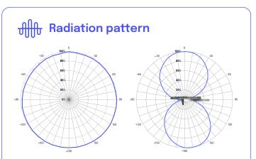
Radiation pattern is heavily affected by the shape of the tagged asset. Testing in real environment is recommended to find the best orientation and location for the tag. i) Description
