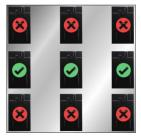
Polarization of **Beontag Heatwave Tough** is as shown below. This should be considered when using linear reader antennas.
